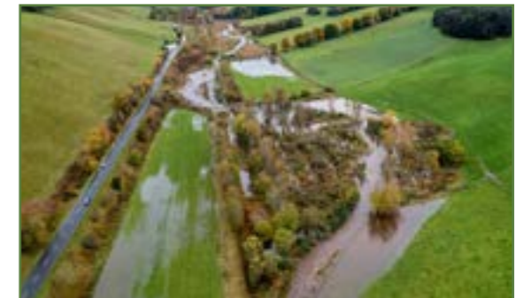
Well-designed riparian woodland and buffer areas holding back water in high flows
